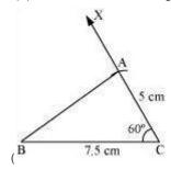
iii) Taking C as centre, draw an arc of 5 cm radius. It intersects CX at point A.
