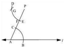
(v) Join P to G to draw a line m. Line m will be parallel to line l.
