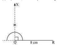
(iii) Taking R as centre, draw an arc of 10 cm radius to intersect ray QX at point P.
