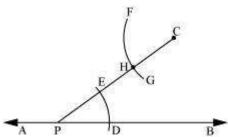
(iv) Adjust the compasses up to the length of DE. Without changing the opening of compasses and taking H as the centre, draw an arc to intersect the previously drawn arc FG at point I.
